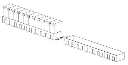
step 3: connect battery cables as below
