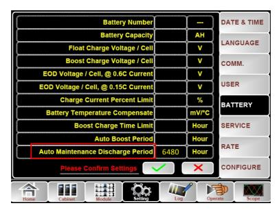
Figure 5-4 Setting period for battery auto discharge
