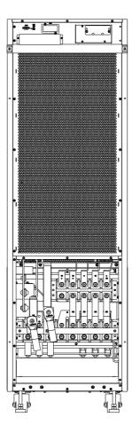
(b) 8 slot UPS Cabinet structure (back view)
