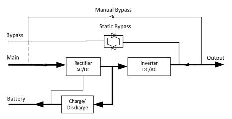
Figure 2-3 UPS conceptual diagram in normal mode
