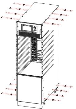
Figure 3-8 Remove bracket for cabinet side door
