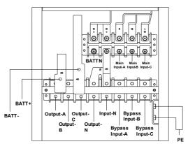
(c) Connections terminals of 8-slot cabinet (dual input)
