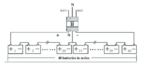
Figure 3-13 Battery string wiring diagram
