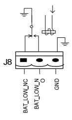
Figure 3-21 Battery warning dry contact interface diagram
