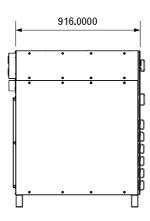
Figure 0-1 Size diagram of 6 module cabinet with PDU
