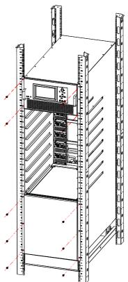
Figure 3-10 Load the UPS into the server cabinet
