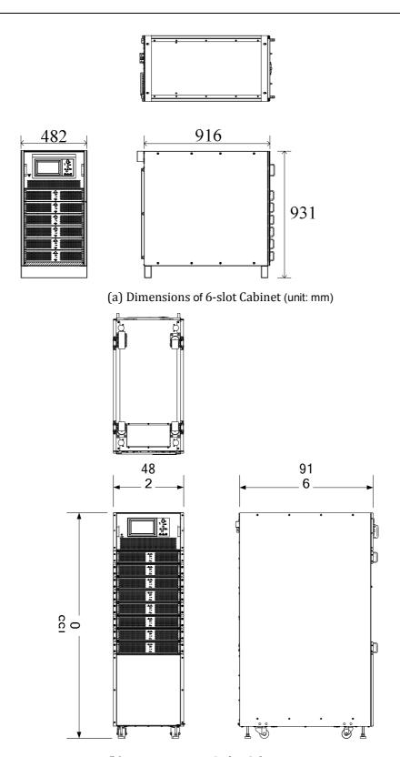
(b) Dimensions of 8-slot Cabinet (unit: mm) Figure 3-1 Dimensions of Cabinet (unit: mm)
