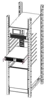
Figure 3-11 Insert module to cabinet
