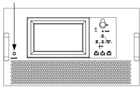
Figure 5-1 the position of the battery cold start button on cabinet
