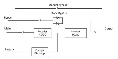
Figure 2-1 UPS Conceptual Diagram
