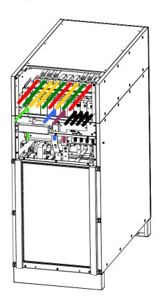
Figure 0-3 PDU Cable entry
