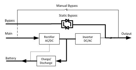
Figure 2-6 UPS conceptual diagram in Bypass Mode
