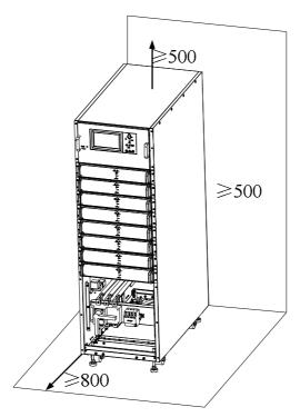
Figure 3-5 Cabinet space reservation schematic (unit: mm)
