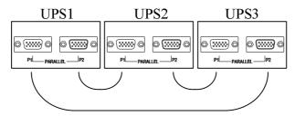
Figure 5-7 Parallel connection
