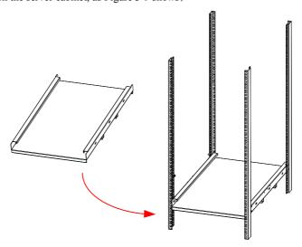
Figure 3-9 Install rack tray
