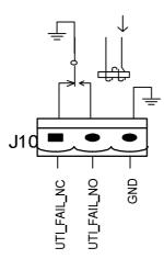
Figure 3-23 Utility failure warning dry contact interface diagram
