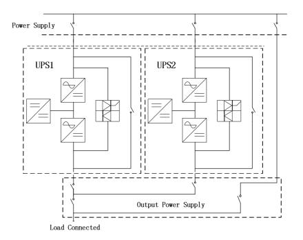
Figure 5-6 Parallel diagram
