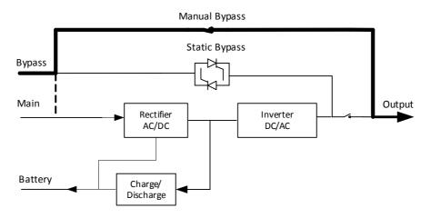
Figure 2-7 UPS conceptual diagram in Maintenance Mode
