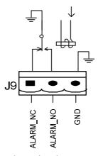
Figure 3-22 Integrated warning dry contact interface diagram
