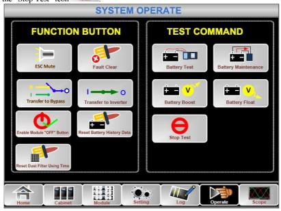
Figure 5-3 Battery maintenance
