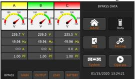
Fig.4-4 Data display page (Bypass)
